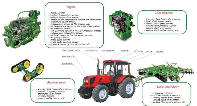
Figure 1: Diagram of the distribution of sensors in the power units of the machine
